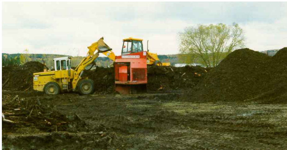
Picture 6: Mechanical screening of wastes by the Town of Penetanguishene
