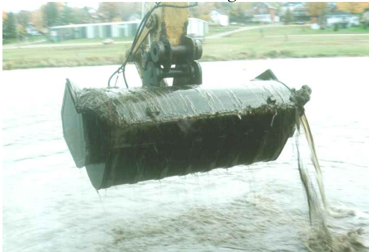
Picture 6: Mechanical screening of wastes by the Town of Penetanguishene
